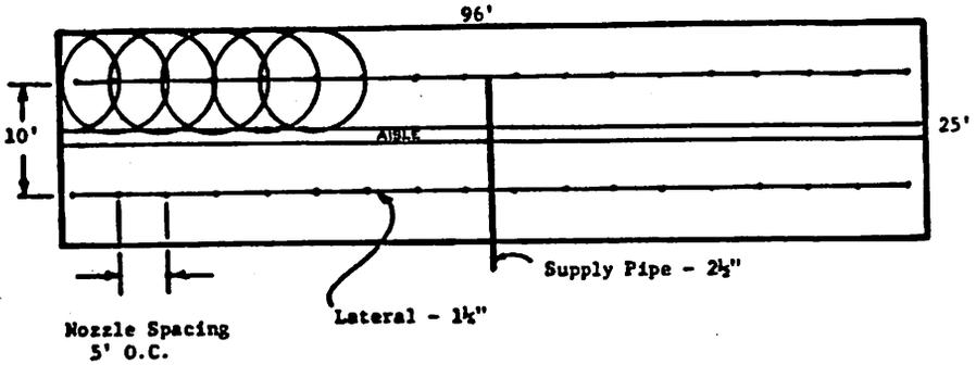
Design using 2 gpm nozzles - whole greenhouse watered at one time.
