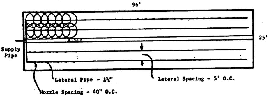
Design using 0.5 gpm nozzles - Each lateral controlled by solenoid and sequenced so one lateral operates at a time.
