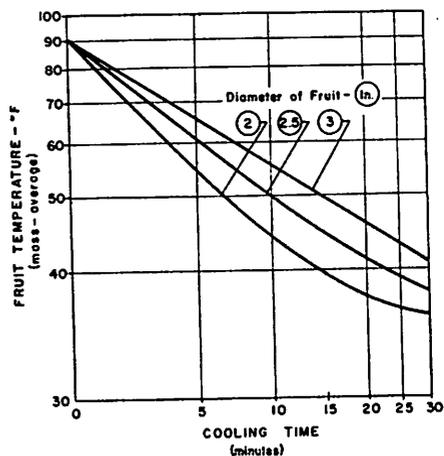
FIGURE 7.—Cooling rate for peaches properly cooled in 35° F. water.
