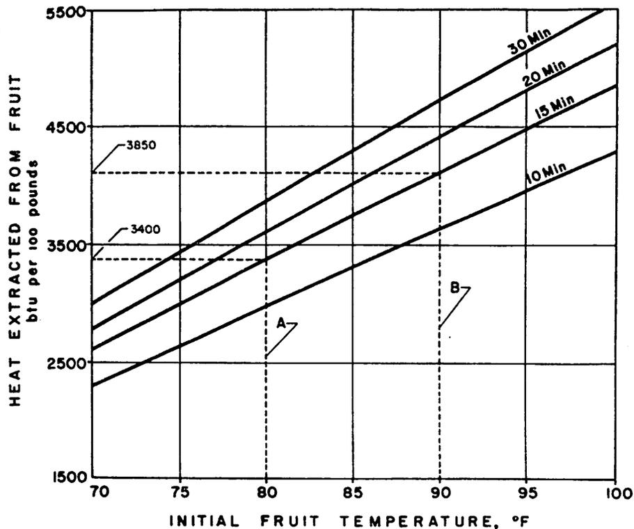
FIGURE 10.—Cooling rate of a 2½-inch-diameter peach of various starting temperatures in 35° F. water. The temperature of fruit entering the hydrocooler determines the cooling load and hence refrigeration requirements.
