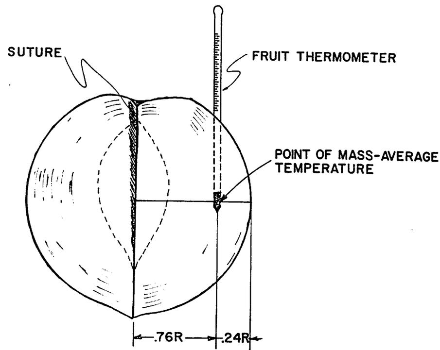
FIGURE 11.—Measuring the mass-average temperature of a peach with a fruit thermometer.
