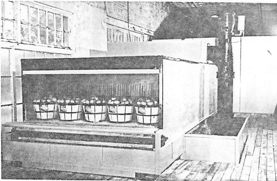
FIGURE 1.—Small conventional flood-type hydrocooler. Fruit is packed before it is placed in the cooler.
