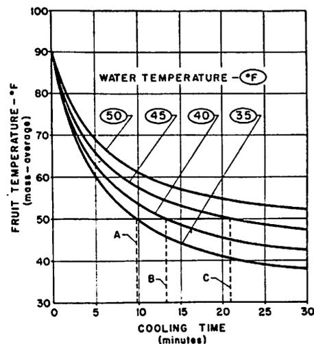
FIGURE 8.—Temperature reduction of 2½-inch-diameter peaches, cooled in water at various temperatures.
