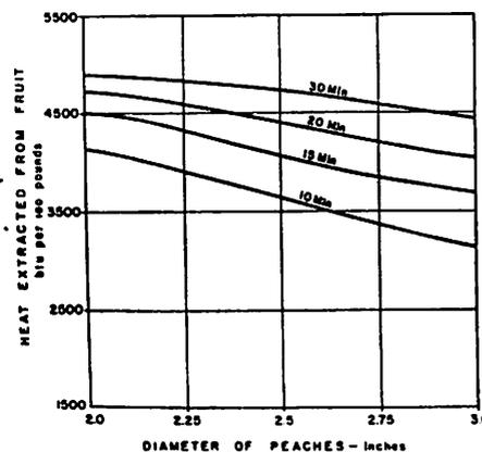
FIGURE 9.—Heat extracted from peaches of specified sizes initially at 90° F., cooled in water at 35° F.
