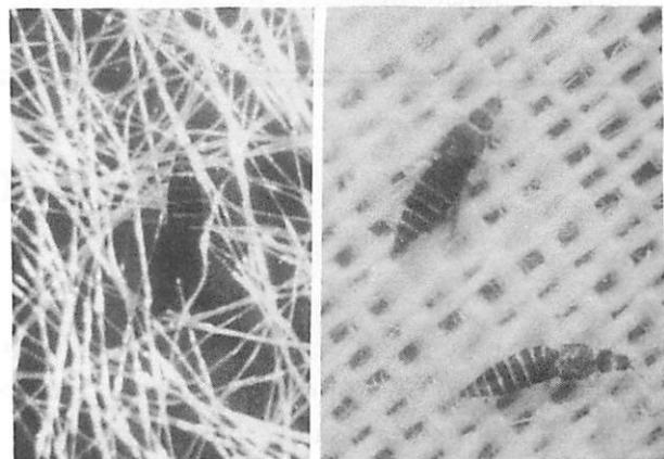
Figure 8. Close up of spunbonded polyester (left) and batiste (right) with a slide of a thrips the same size as the western flower thrips.
