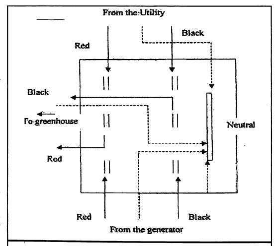
Figure 1. Emergency generator switch diagram. Double pole-double throw switch. Neutral lines go to a common bond. If three phase power is used a triple throw-double throw switch is needed.
