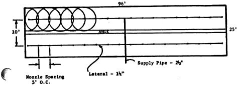
Design using 2 gpm nozzles - whole greenhouse watered at one time.
