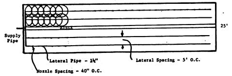
Design using 0.5 gpm nozzles - Each lateral controlled by solenoid and sequenced so one lateral operates at a time.
