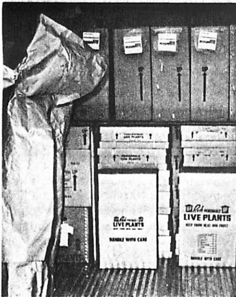
An example of decking - a method carriers use to protect their foliage shipments.
