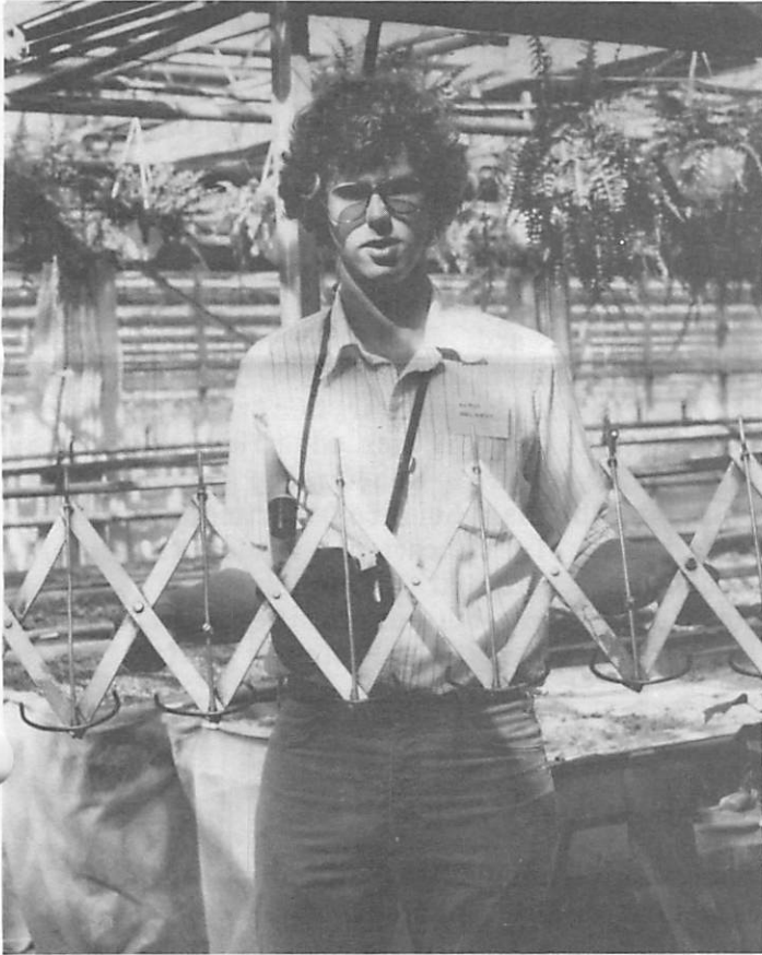
Figure 4: Pot spacer held by Bill Miller -- to pick up pots at one spacing and by moving handles place pots down at a different spacing. Photographed at Westland Greenhouses.
