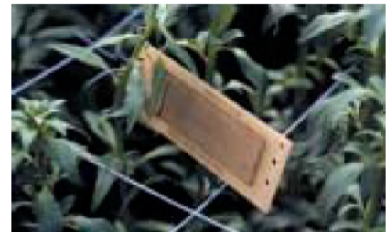
Leaf wetness sensor in commercial snapdragon field.
