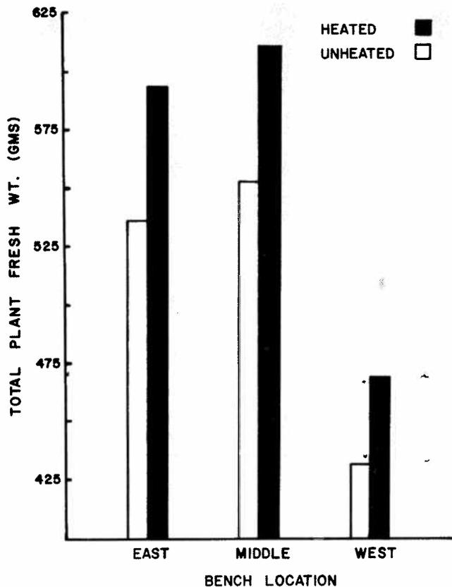
Figure 6: Total fresh weight of 'White Sim' carnation plants harvested 26 weeks after a November 18, 1975, planting. No significant difference at 5% level.
