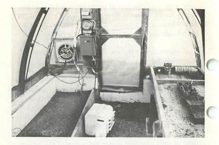
4. A third system utilizing two 1.5 KW quartz tube infrared heaters and two 1 KW soil heating cables gave the best results for germination and starting plants. Air temperature sensing thermostats were used to control the temperature. The infrared heaters were located below the ridge at a height of 6 1/2 feet from the ground and heating cables were buried in the benches. Heating costs per year were approximately \$63.00.
