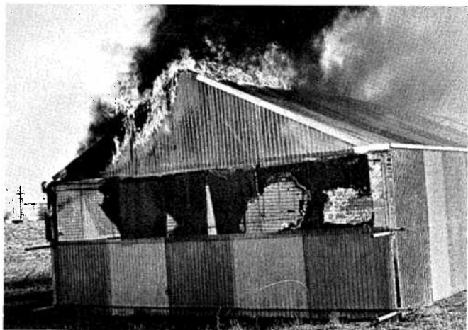
Figure 1. Controlled fire started in cooling pad area and jumping PVC barriers of 6", 12", and 24" in a 12 mph artificial wind.
