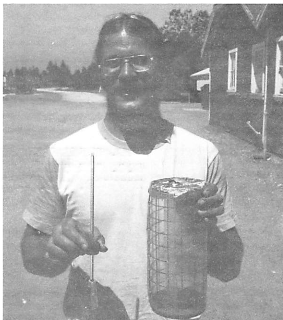
Fig. 1. Local plant expert Dennis Suit holding a cylinder assembly used for evaluating films. It is 10 inches long and 4 inches in diameter with \frac{3}{4} -inch plywood ends and sidewalls of 1-inch steel mesh. Cylinder shown is covered with clear polyethylene. Thermometer bulb is shielded to prevent direct absorption of sunlight.
