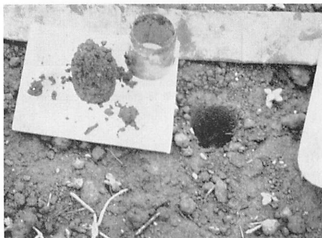
Figure 3: Soil core, empty coring tool and hole made in process of removing sample.
