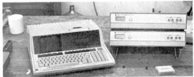
Fig. 6: The HP-85 Desk Computer with two digital acquisition and control units to be programmed for environmental control in the two houses.
