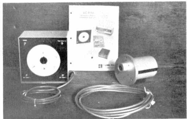
Fig. 7: One of the two infrared thermometers for remote plant temperature sensing. The unit in the west house will be used for temperature control. Four aspirated air temperature sensors will be averaged for temperature control in the east house. One of these $2600 units was donated by Raytek, Inc.
