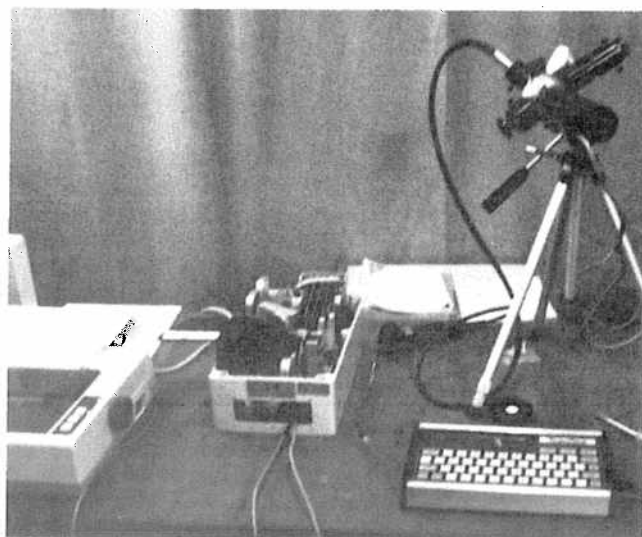
Fig. 1: LI-COR's digital spectroradiometer for measuring spectral energy at different wavelengths. An integration sphere is mounted on the tripod which allows measurement of reflectance and transmittance. A printer is on the left. This equipment can be taken to the field.
