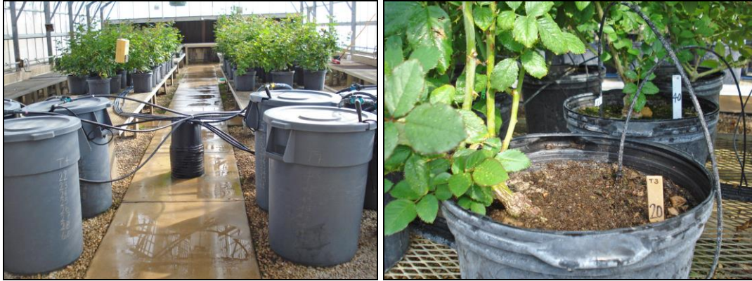
Figure 1. Layout of cation ratio study. The nutrient solutions from the tanks are delivered, via submersible pumps, to the plants through an irrigation manifold, with one calibrated spot-spitter (emitter) per pot.
