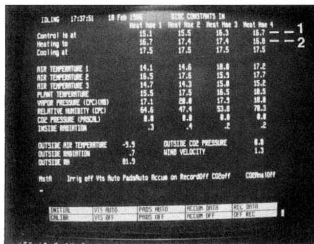
Fig. 4: Typical display on CRT showing conditions in each house. This display is refreshed each time the system executes (every 60 sec.), and some time is required to interpret what the operator sees. Item "1" is the average air temperature from 3 stations in the house. Item "2" is the re-calculated setpoints for heating and cooling which are compared to "1" for control purposes. Temperatures on this display are in degrees Celsius, vapor pressures in millibars and CO 2 levels in Pascals. The bottom line shows which houses are being watered, misted or injected with CO 2 . The remaining, reversed display (black on green) refers to single stroke keys which the operator can use to control the system (i.e., manually water, turn off CO 2 , turn mist on manually, accumulate data, call programs, etc.).
