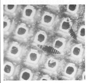
Figure 7. Close up of Vispore with a slide of a thrips the same size as the western flower thrips.
