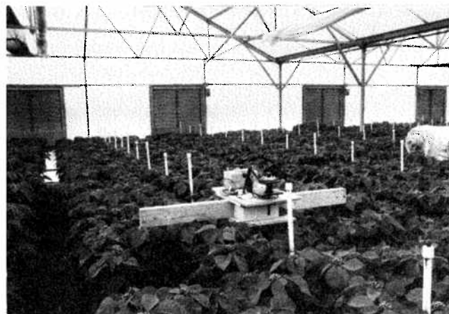
Fig. 2: Typical placement of radiation measuring equipment in a commercial greenhouse range.
