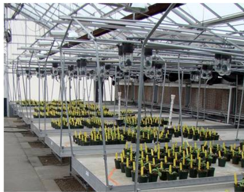
Figure 1. Light-emitting diodes (LEDs) were used to deliver night-interruption lighting. The LEDs emitted different ratios of red and far-red light on each bench, and results were compared to those under incandescent lamps.
