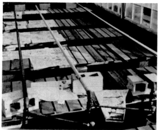
Fig. 1: Arrangement of heating pipe for measuring heat transfer as a function of external surface
